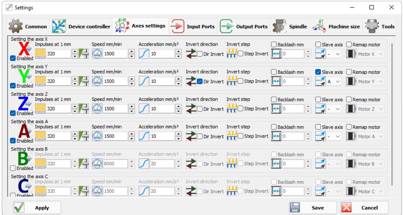
Set the required number of pulses for each axis. If necessary, specify the subordination of the axes and change the direction of movement.
