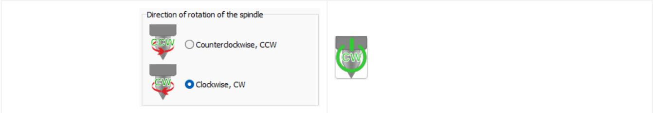
If you have configured the output ports "Spindle CCW" and checked "Counterclockwise, CCW", then the button "Turn the spindle" is labeled "CCW".
