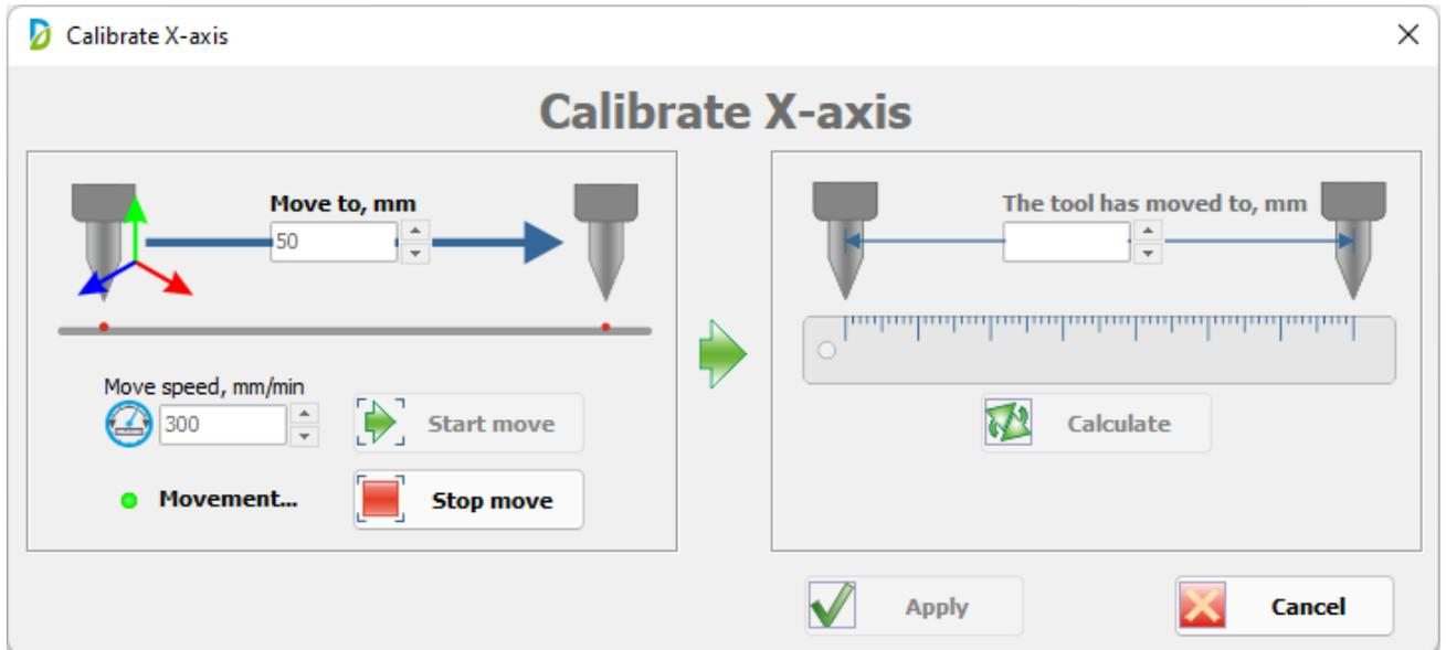
After the tool has finished moving, use the ruler to measure the actual distance the tool moved. Enter this value in the “The tool has moved” to field.
