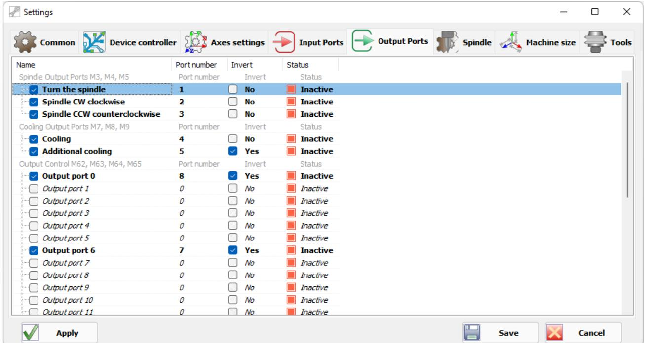
Set the output port numbers according to the configuration of the machine and the CNC controller.
