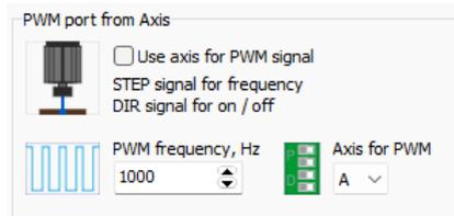
Set the checkbox "Use axis for PWM signal", select "Axis for PWM" and set the maximum frequency in the input field "PWM frequency, Hz".
