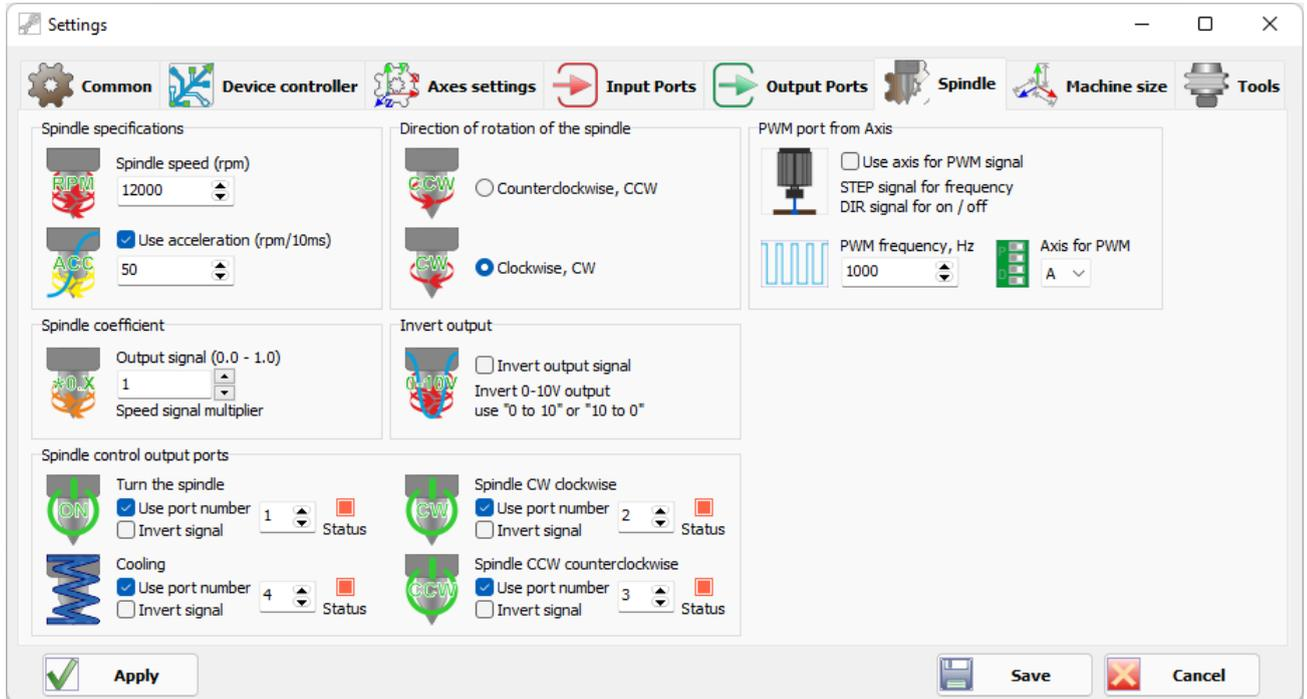
Set the speed and acceleration parameters according to the spindle specification. Set the default spindle rotation direction.
